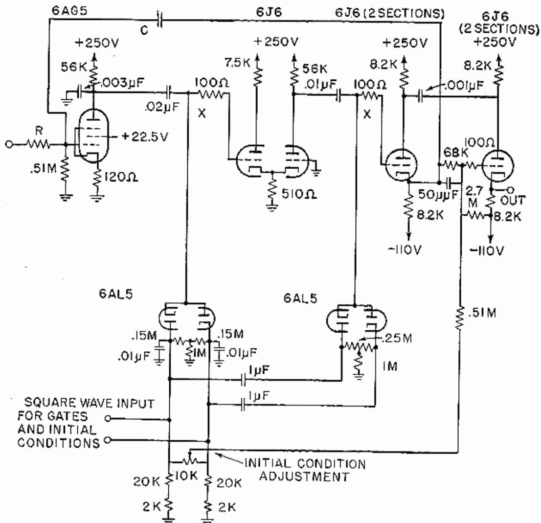
FIG. 8.7. Circuit diagram of an integrator from the MIT repetitive computer. Note the clamping circuits, used to discharge the integrating capacitor, and the summing circuit, used to add initial condition voltages to the integrator output voltage. The initial condition voltage is *not* used to charge the integrating capacitor directly in this arrangement.
